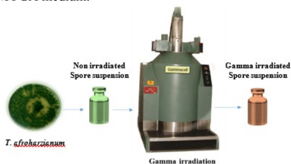
Fig 1. Gammacell 220 irradiator used to induce mutation in Trichoderma afroharzianum NAS107
